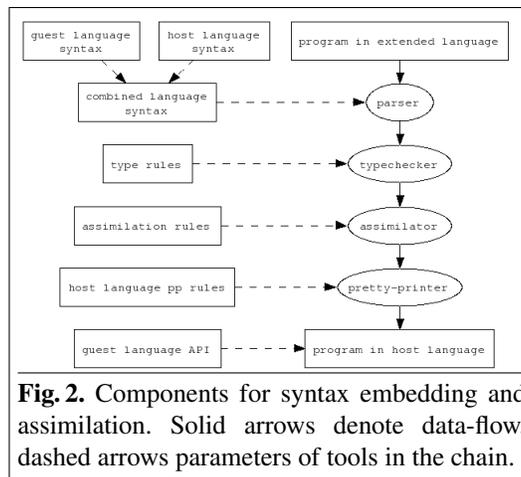
**Fig. 2.** Components for syntax embedding and assimilation. Solid arrows denote data-flow, dashed arrows parameters of tools in the chain.
